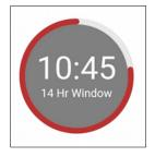
The bottom center clock displays the remanining duty time in the *14 Hour Shift Window*.
